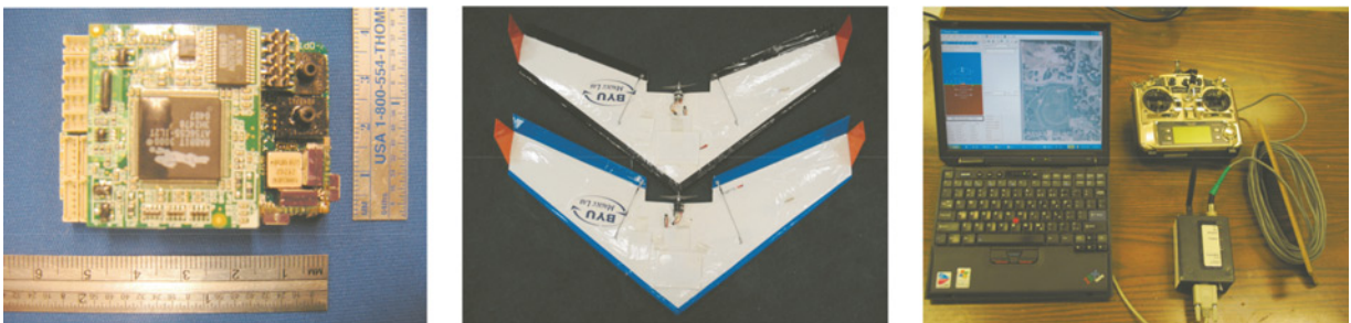
Fig. 5 (a) Kestrel autopilot, (b) Unicorn airframes, (c) ground station components.
